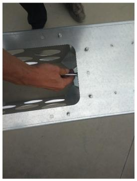
• Finally, the nuts of the mounting corners can be tightened with a socket wrench.
