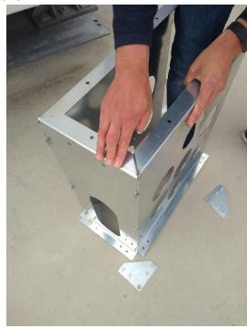
• Take the last front panel and use the grooves to mount the panel to the two side panels.
