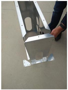
• This makes sure the four panels are joined together. They still need to be secured using the mounting corners. Carefully tilt the anchor to slide the mounting corners into position. The mounting corners can be fixed by hand tightening the supplied nuts.
