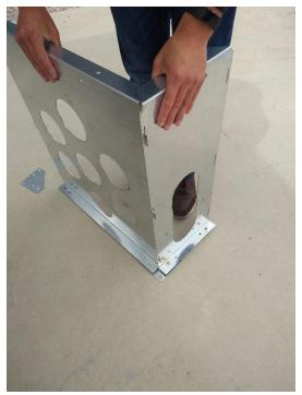
• Take the second side panel and place this in the same position as the other side panel. Use the grooves to join the side panel to the front panel.
