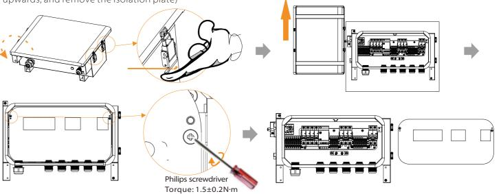
d) Mount X3-Matebox on bracket A and tighten the screws.
