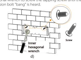
Step 4: Finally, install X3-Hybrid G4 inverter bracket; (Please refer to X3-Hybrid G4 inverter quick installation guide).
