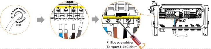
4) Pass the PV /Gird line through the PV port of The X3-MateBox, and then find PV(PV1+/PV1-/PV2+/PV2+) and Grid(N/R/S/T) port inside the X3-Matebox. Force the wire harness directly into the hole to jam, gently twist not to loosen.
