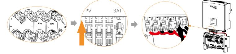
$\times$ Note: X3-Hybrid-5.0-M and X3-Hybrid-6.0-M inverters have only two MPPT and two PV strings, so when connecting, you need to unplug 1/2 of the PV in the X3-Matebox.
