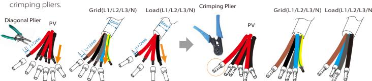
b) Gird(PE) strip the grounding cable insulation(lenhth"L), insert the stripped cable into the R type terminal, and then clamp it
